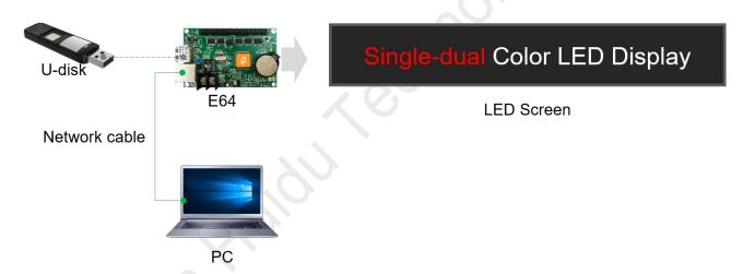
2. Supports LAN control, and can be wirelessly controlled via the "LedArt APP" through LAN connection.
