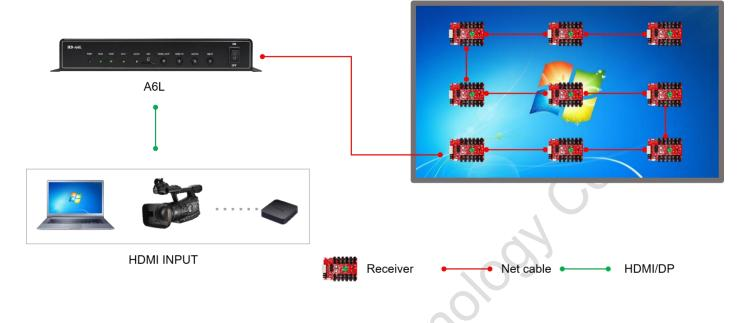
3. Synchronous control, through HDMI signal input, synchronous playback.
